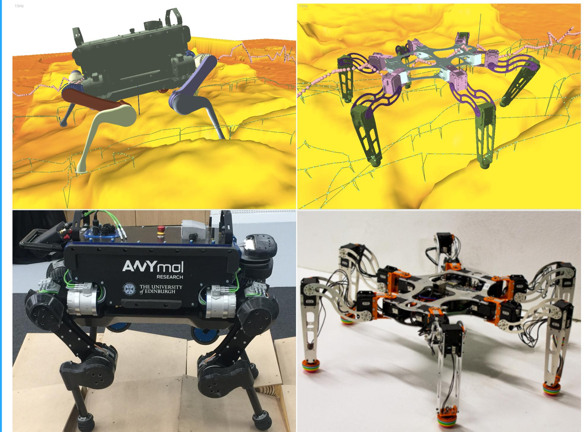
The goal of this research is to plan feasible paths for legged robots walking on irregular terrain, taking into account motion constraints (collisions, static stability, robot workspace) in high-dimensional search space.
