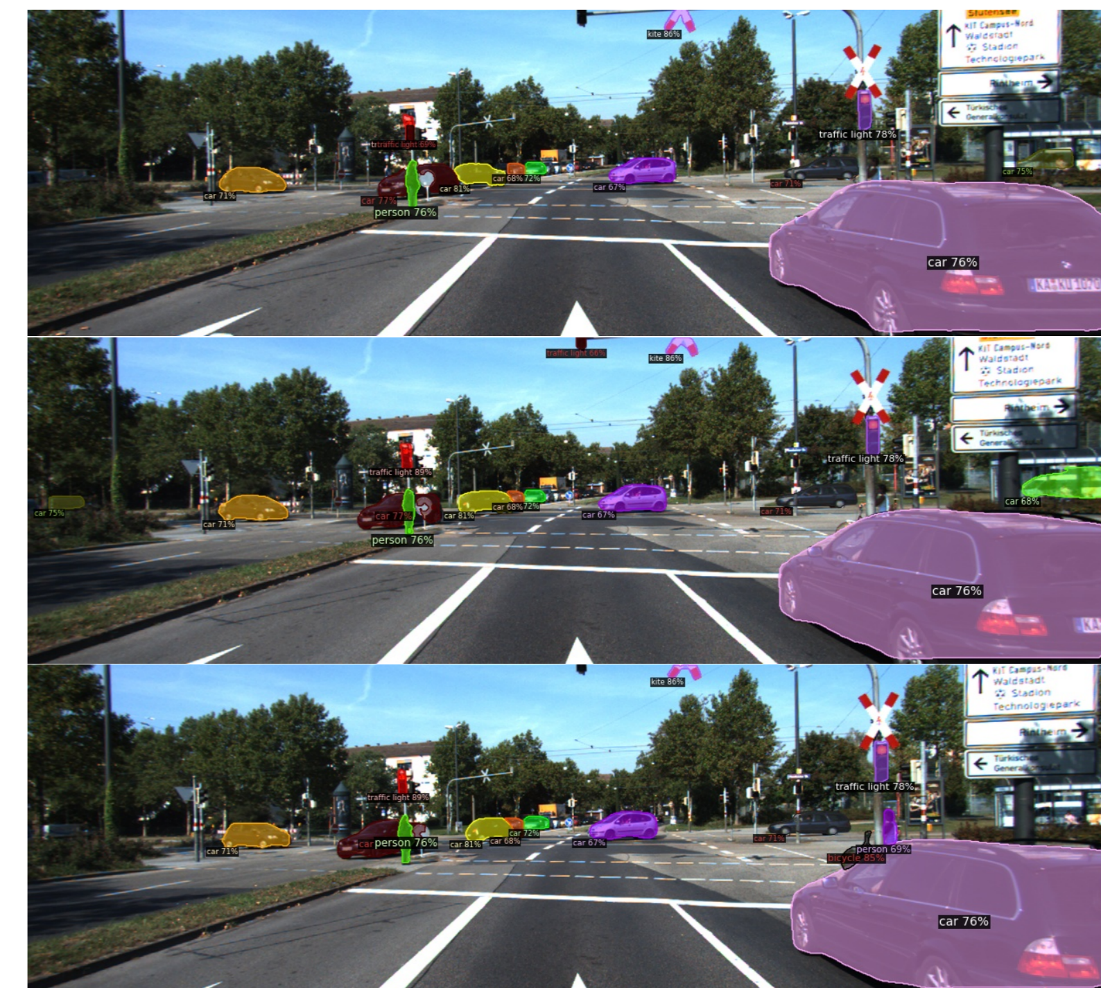
Figure 3: Tracker visualisation on subsequent frames of a test sequence.
