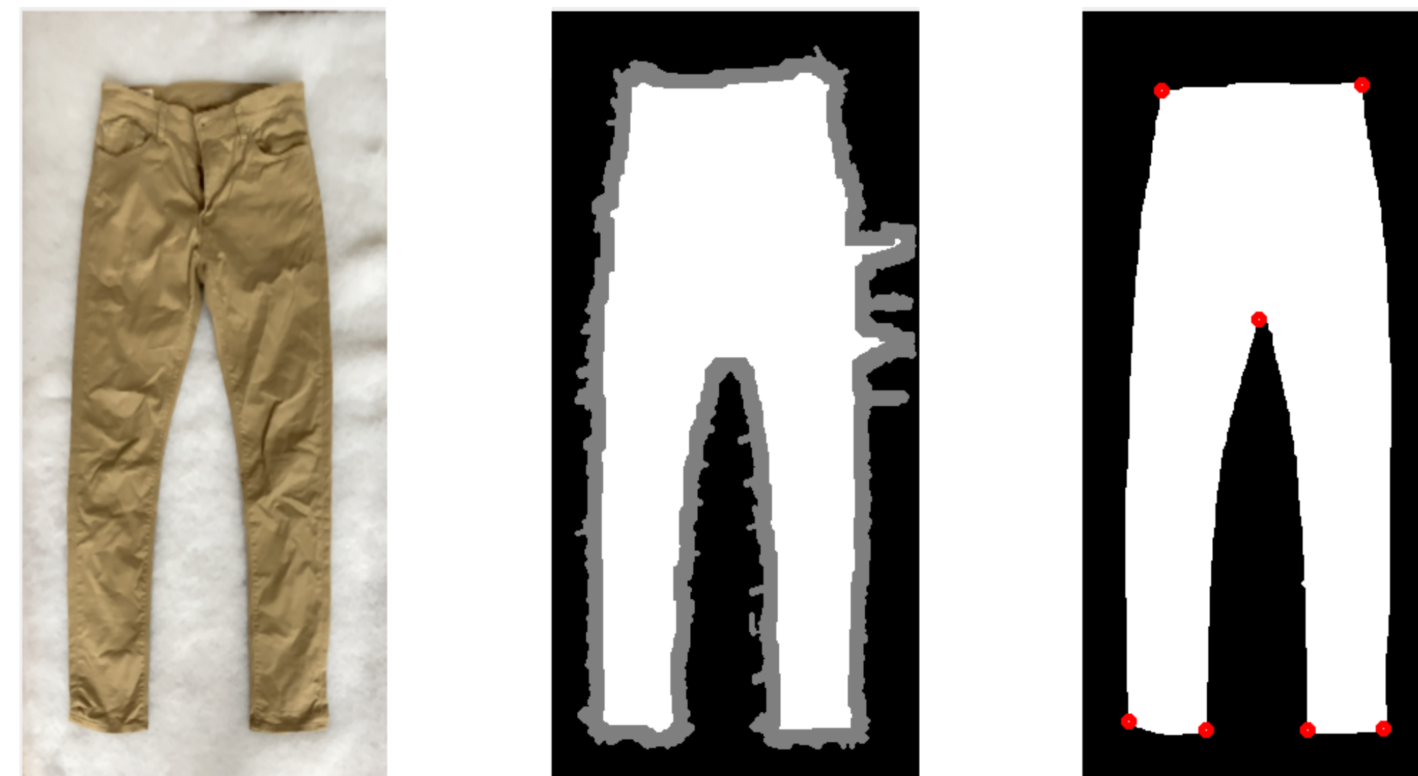
Figure 2: Left: original image. Middle: initialisation mask obtained with edge detection, contour filling and erosion (black means background, gray probable background, white probable foreground). Right: final segmentation with Grabcut and keypoints.
