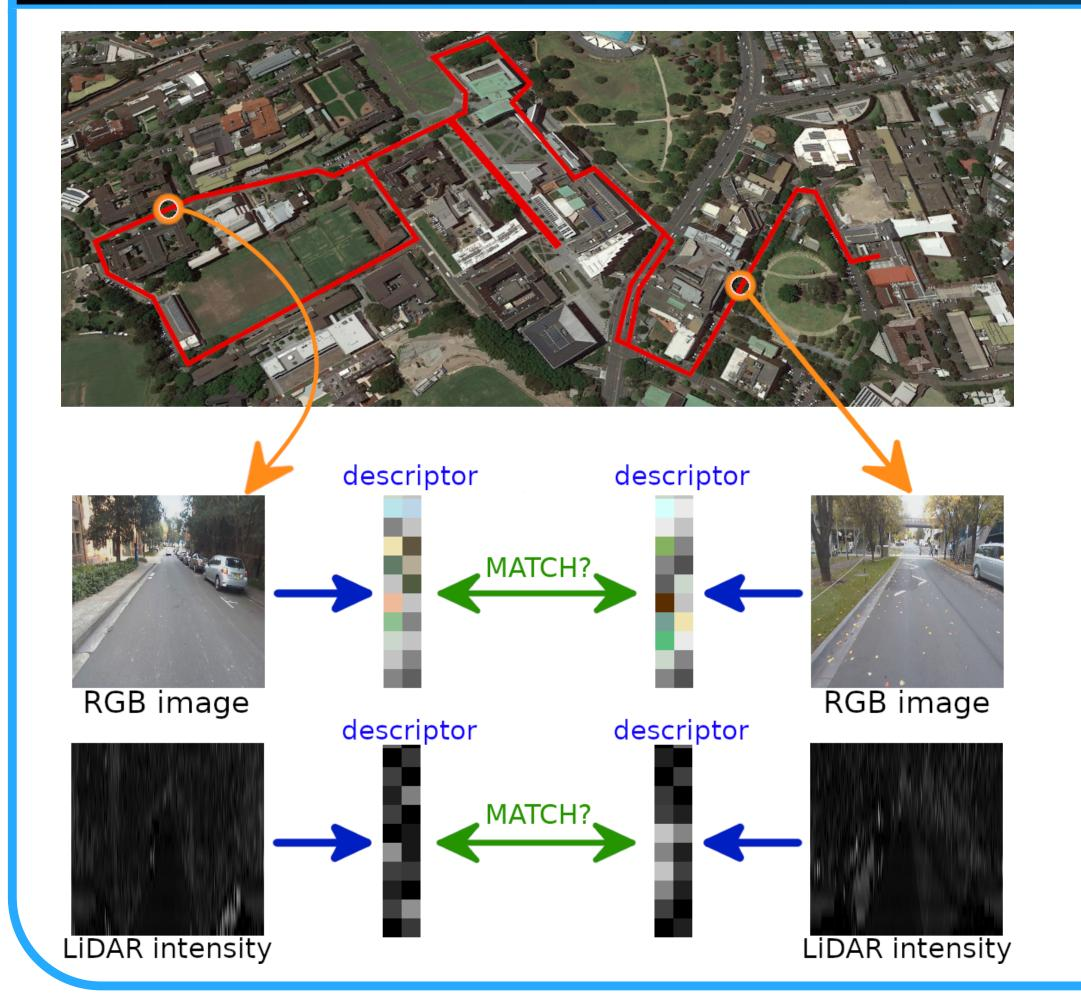
This research focuses on a place recognition task - checking if the data received from the sensor corresponds to a known location, to reduce drift and provide global localization. Known flaws of camera-based solutions and increasing LiDAR popularity lead to the following questions:
